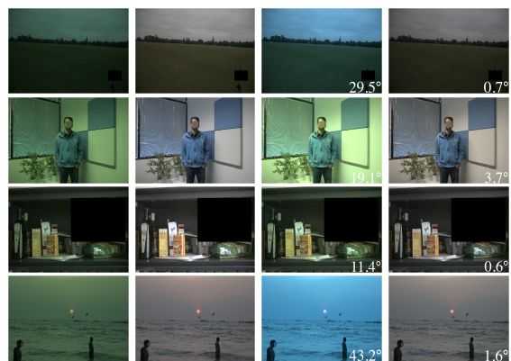
Figure 10: Random worst case examples from global datasets. (First two rows: Left-to-right) Input, ground truth, the result of double-opponent cells based color constancy and proposed method with double-opponent cells based color constancy. (Last two rows: Left-to-right) Input, ground truth, the result of white-patch Retinex and proposed method with white-patch Retinex. Errors are given at the bottom right corner of the images.
