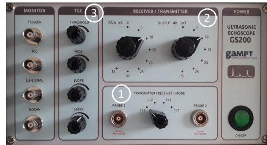
Abb. 6: Bedienfeld des Ultraschallgeräts mit 1: Transmitter | Receiver - Mode, 2: Receiver | Transmitter, 3: Time-Gain-Control (TGC).
