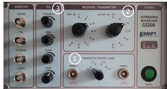
Abb. 6: Bedienfeld des Ultraschallgeräts mit 1: Transmitter | Receiver - Mode, 2: Receiver | Transmitter, 3: Time-Gain-Control (TGC).
