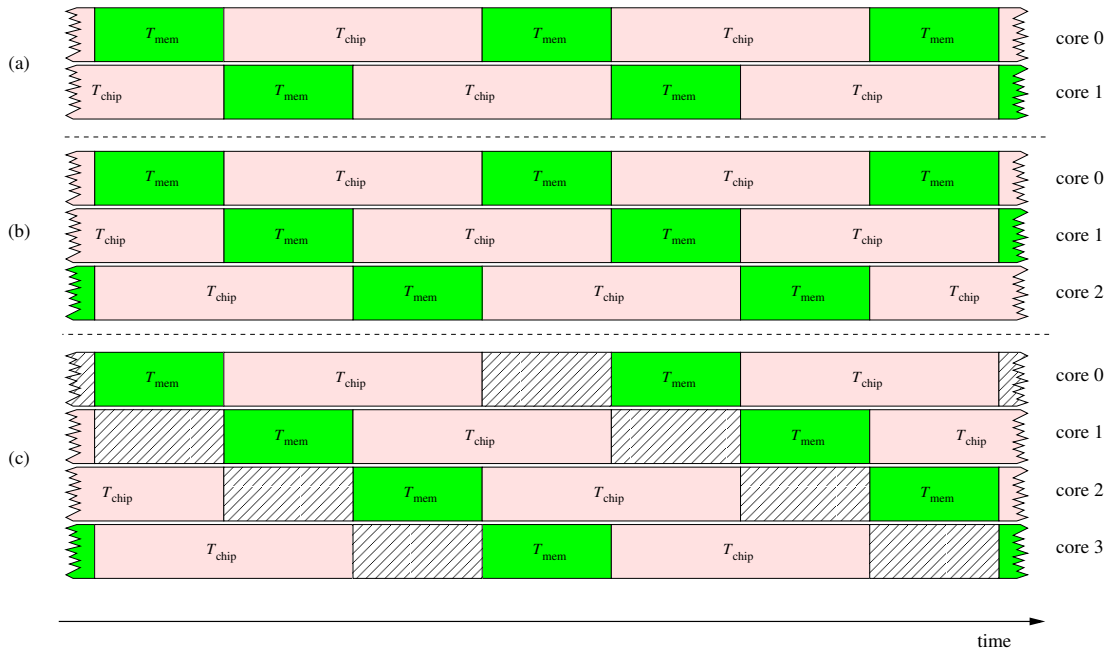
Figure 3.6: ECM model multicore scaling and saturation on a chip with a memory bandwidth bottleneck. T_{chip} is the time for running the loop with data from scalable resources, while T_{mem} is the memory transfer time. In this example we assume T_{chip}/T_{mem} = 2 . (a) With two cores, memory access is not a bottleneck and scalability is perfect. (b) Three cores are needed to saturate the memory interface. (c) Beyond three cores, performance does not increase since the bottleneck is exhausted. This results in idle phases (hatched boxes).
