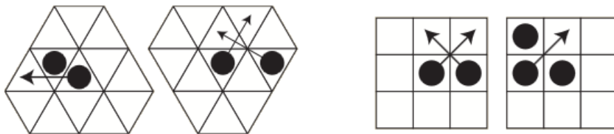
Figure 3.5: Forbidden moves by using the Moore neighborhood in triangular and rectangular grids [4]
